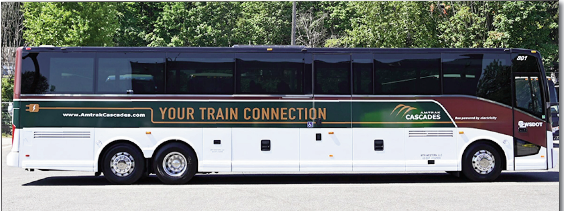
The new full size electric bus can make its 200 mile daily run on one charge. (Amtrak photo)
